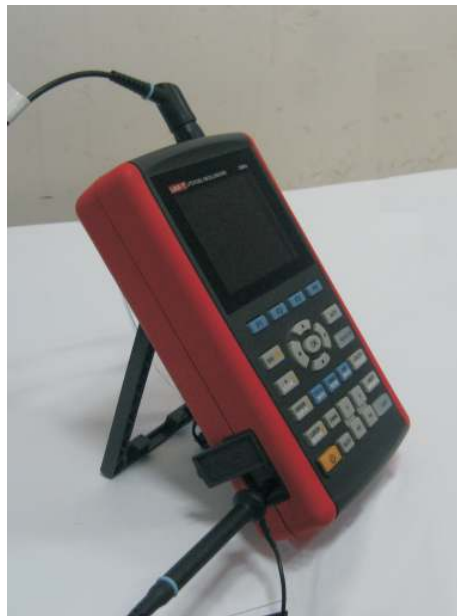
Figure 3-2 Compensation Output Connection
