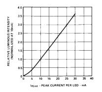
Figure 13. Relative luminous intensity vs. DC forward current
