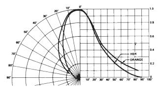
Figure 6. Relative luminous intensity vs. angular displacement
