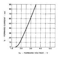
Figure 2. Forward current vs. forward voltage
