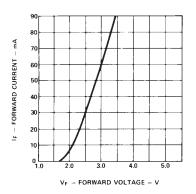
Figure 12. Forward current vs. forward voltage
