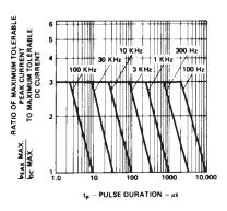
Figure 5. Maximum tolerable peak current vs. pulse duration. (I<sub>DC</sub> MAX as per MAX ratings)
