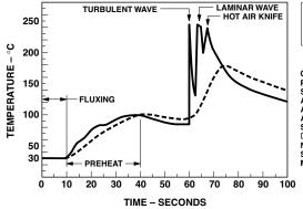
TOP SIDE OF D PC BOARD CONVEYOR SPEED = 1.83 M/MIN (6 FT/MIN)□ PREHEAT SETTING = 150°C (100°C PCB)□ SOLDER WAVE TEMPERATURE = 245°C□ AIR KNIFE AIR TEMPERATURE = 390°C□ AIR KNIFE DISTANCE = 1.91 mm (0.25 IN.)□ AIR KNIFE ANGLE = 40°□ SOLDER: SN63; FLUX: RMA□
