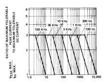
Figure 15. Maximum tolerable peak current vs. pulse duration. (I<sub>DC</sub> MAX as per MAX ratings)
