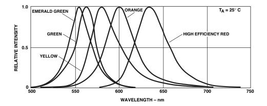
Figure 1. Relative intensity vs. wavelength
