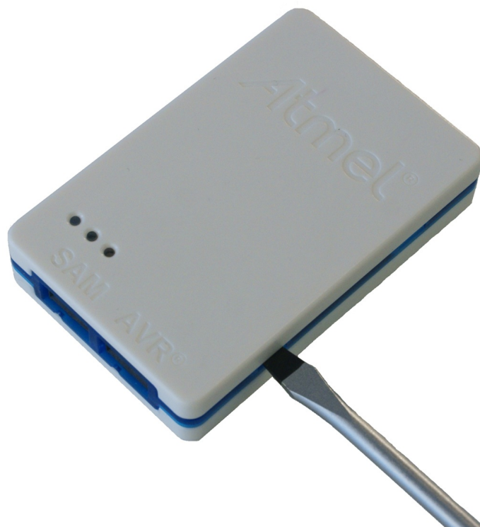
Figure 2-13. Opening the Atmel-ICE (2)
