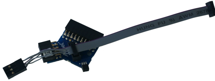
Figure 2-10. Atmel-ICE AVR Probe Connection
