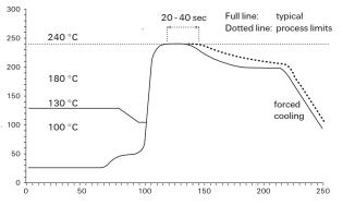
Resistance to soldering heat - Reflow profile
