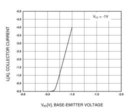
Figure 3. Base-Emitter On Voltage
