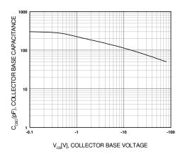
Figure 4. Collector-Base Capacitance
