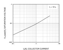
Figure 2. Collector-Emitter Saturation Voltage
