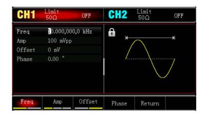
Press Freq soft key to set the frequency, use numerical keyboard to input 2 and then select the unit of parameter to kHz;
