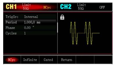
Burst (period of pulse string) is only for N cycle mode, which means the time from one pulse string to the next pulse string. When trigger source is external, burst (period of pulse string) option in parameter list will be hidden. The range of burst (period of pulse string) can be set to 1µs~500s; the default range is 1.001ms. After the type is select N cycle, it can be change by multifunction rotary knob and arrow keys or press soft key Burst to complete the setting.
