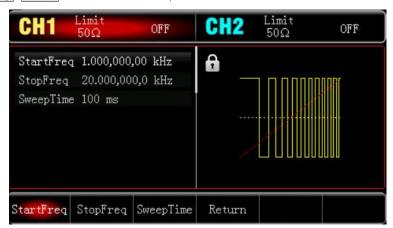
Press Start or Stop soft key, use numerical keyboard to input 1 and then select the unit of parameter to kHz.
