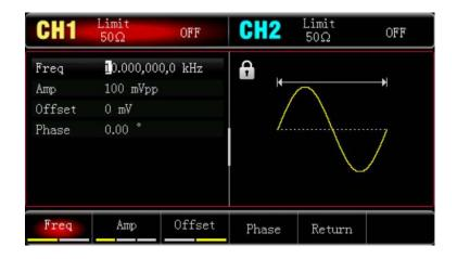
Press Freq soft key to set the frequency, use numerical keyboard to input 10 and then select the unit of
