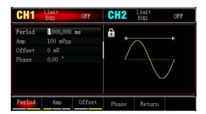
Press the corresponding soft key to set a parameter, to input numerical value and then select the unit.
