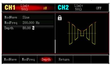
To view the shape of the AM through an oscilloscope as shown in the following figure.
