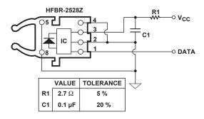
Figure 11. Recommended receiver application circuit
