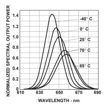
Figure 3. Typical normalized optical spectra
