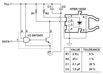
Figure 6. Recommended transmitter drive circuit ( $I_{E,n} = 60 \text{ mA nominal at } T_A = 25^{\circ}\text{C}$ )
