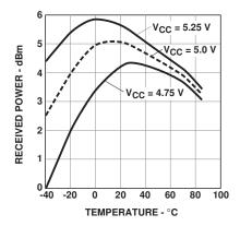
Figure 7. Typical POF receiver overdrive,  $P_{\rm RL,max'}$  at 10 MBd, vs. temperature and power supply voltage
