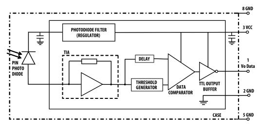
Figure 12. HFBR-2528Z receiver block diagram
