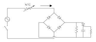
Ct2 Test capacitance [µF] Imax2 Max current across the NTC under test [A] Number of cycles: 1000
