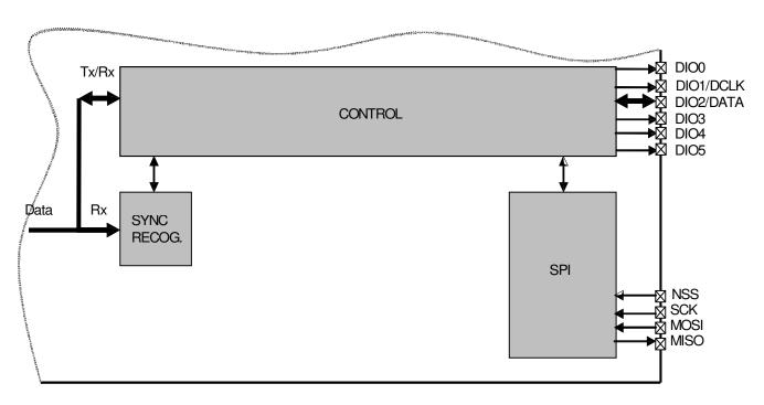
Figure 28. Continuous Mode Conceptual View
