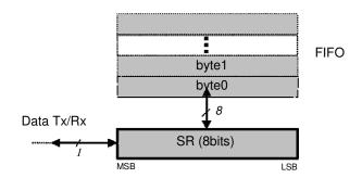
Figure 25. FIFO and Shift Register (SR)
