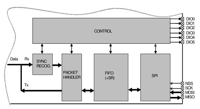
Figure 31. Packet Mode Conceptual View
