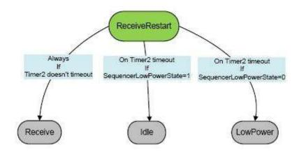
Figure 19. Sequencer Transitions From ReceiveRestart State
