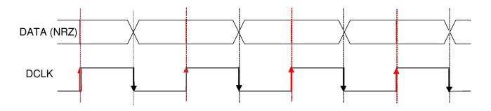
Figure 30. Rx Processing in Continuous Mode
