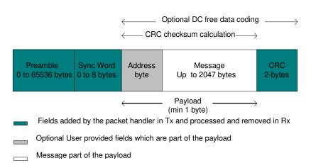
Figure 32. Fixed Length Packet Format
