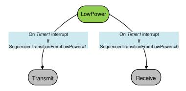
Figure 17. Sequencer Transitions From LowPower State
