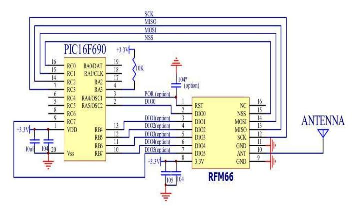
Figure 41:+20dBm Schematic
