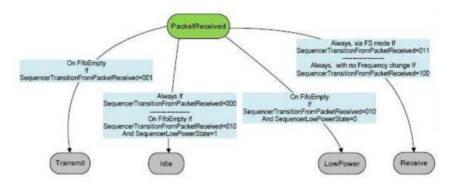
Figure 20. Sequencer Transitions From PacketReceived State
