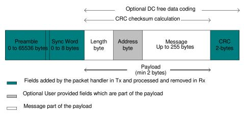
Figure 33. Variable Length Packet Format
