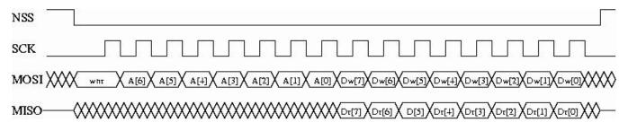
Figure 24. SPI Timing Diagram (single access)
