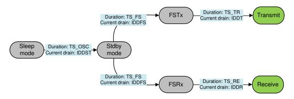
Figure 15. Startup Process
