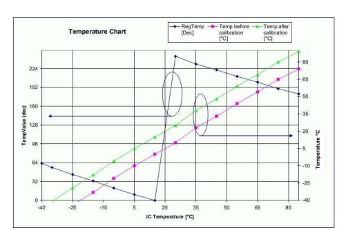
Figure 14. Temperature Sensor Response
