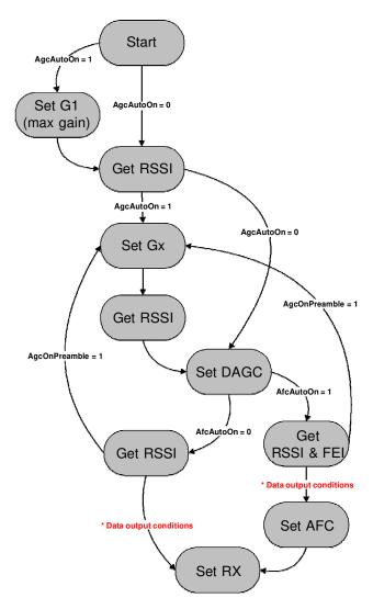
Figure 9. Receiver Startup Process.
