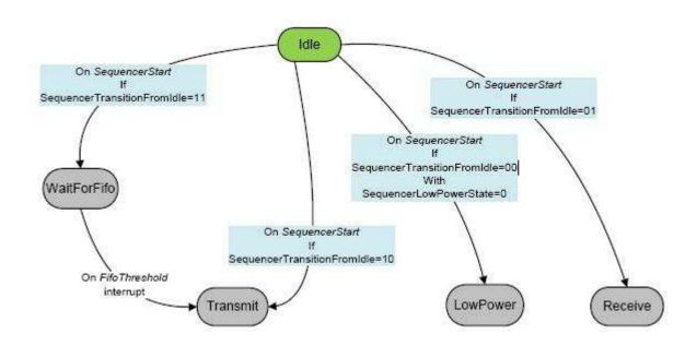
Figure 16. Sequencer Transitions From Idle State
