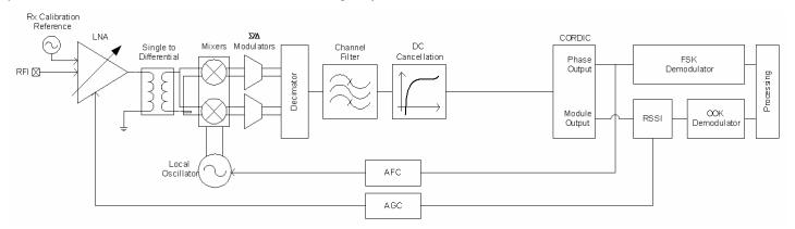
Figure 8. Receiver Block Diagram
