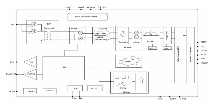
Figure 4. Simplified RFM66 Block Schematic Diagram
