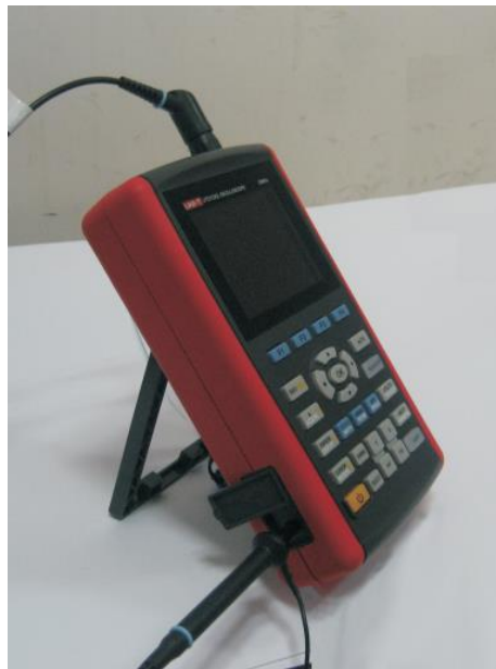
Figure 3-2 Compensation Output Connection
