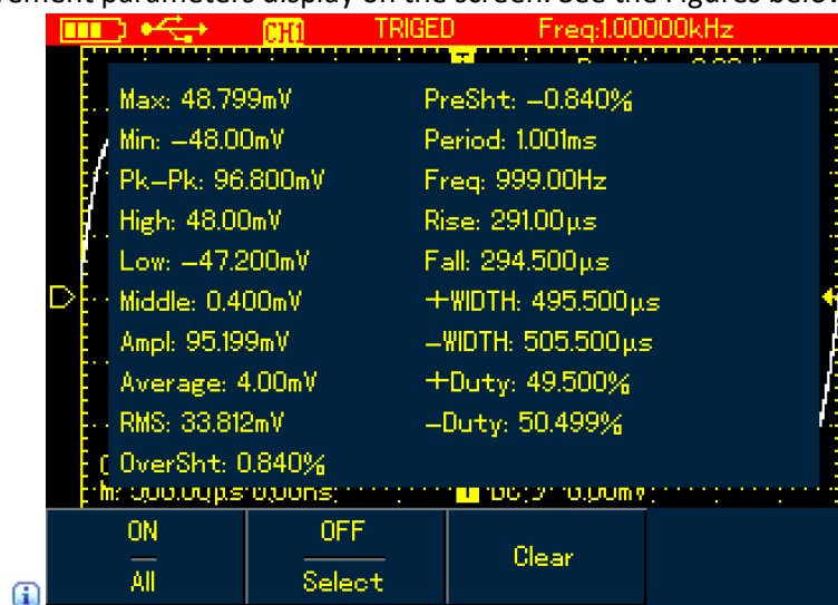
Figure 6-16A UTD1000CL measures all parameters
