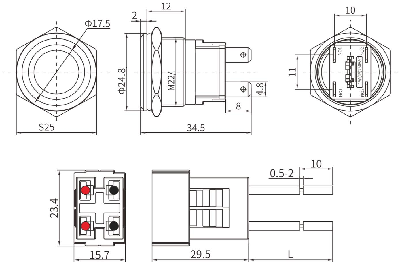
Connector: Cable length: 150mm, 1.5mm<sup>2</sup>
