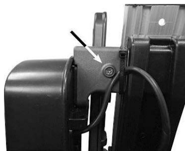
Figure 2: Installation of the rear lights
