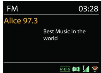
To full scan, press “**INTRO**” remote key. The frequency display starts to run and scans the FM full band.
