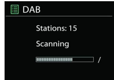
To start a scan manually, choose Full scan. To scan only stations with good signal strength, select Local scan.
