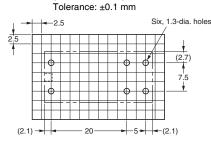
**Terminal Arrangement/ Internal Connections** (BOTTOM VIEW)
