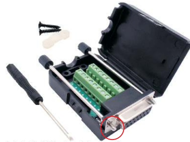
2010C253 - Female connector with locking screw connection
