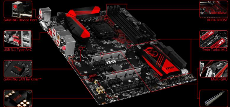
**MSI GAMING LAN POWERED BY KILLER™** MSI GAMING LAN is powered by the Killer<sup>™</sup> LAN E2400 Network Controller featuring intelligent AES 2.0 to automatically prioritize games above other applications. GAMING LAN uses LAN Protect with 15KV anti-surge protection for safety, highlighted with a red LED in the LAN port.
