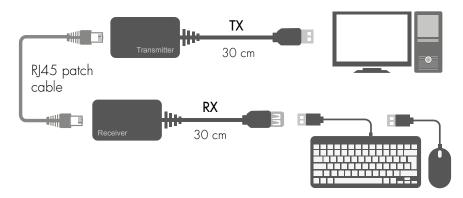
» Extends the distance of keyboard/mouse and other USB devices from an USB-enabled computer
