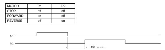
It is necessary to take more than 100 ms intervals for on / off timing between driving Tr1 and Tr2. If the interval is less than 100 ms, an excessive current happen to flow to the relay contacts.
