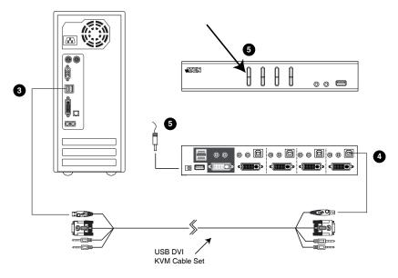
4. At the other end of the USB DVI KVM cable set, connect the USB Type B connector to the Type A USB port in the Port 1 KVM section.
