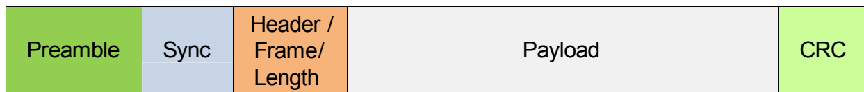
Figure 12. Packet Handler Structure
