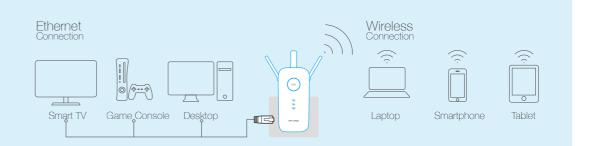
connect the extender to your Ethernet-only device via an Ethernet cable.
