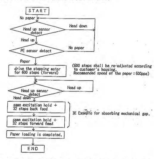
X If recording paper is skew, drive the stepping motor until the paper becomes straight,
