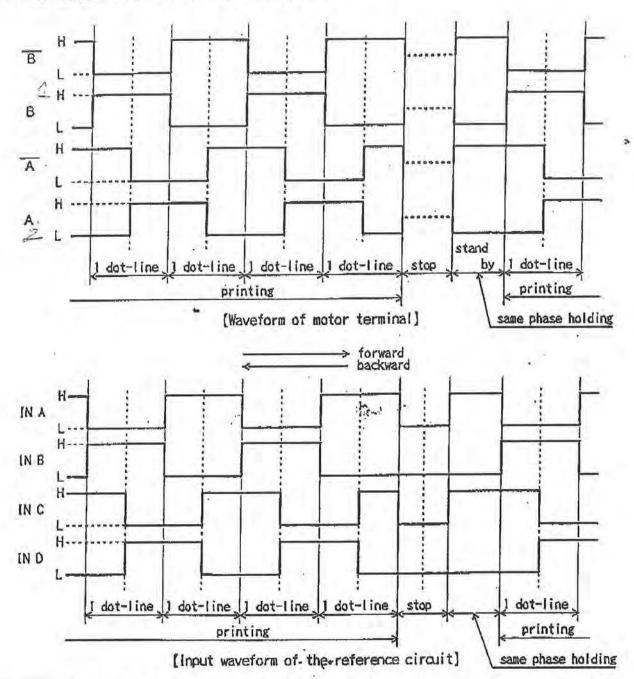
\* Dot-line/Motor step ratio: 1 dot-line/2 steps.
