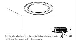
6. Switch on the power and test the light.
