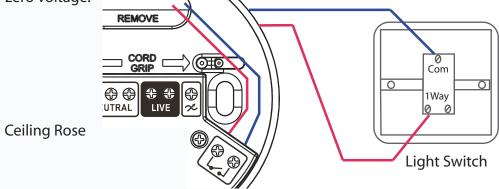
5:Make sure all the cables are connected correctly and securely fastened.
