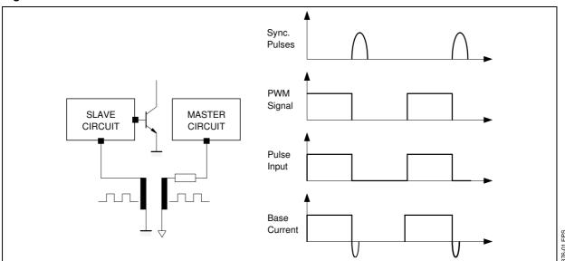
Figure 2: Burst Mode Operation
