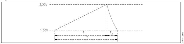
$C_{\rm O}$  capacitor is charged with a constant current. The current is fixed by  $R_{\rm O}$  which is supplied by voltage  $V_{\rm REF}.$
