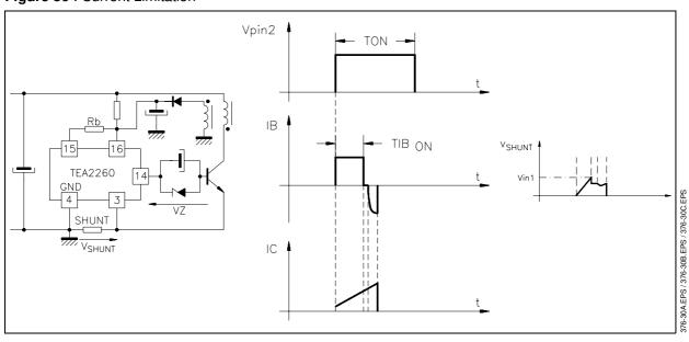
**Note**: in current limitation TIBon  $< T_{ON}$
