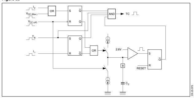
$V_{CC}(off)$  is a signal coming from a comparator checking  $V_{CC}$ . When  $V_{CC} > V_{CC}(stop), V_{CE}(off)$  is high.
