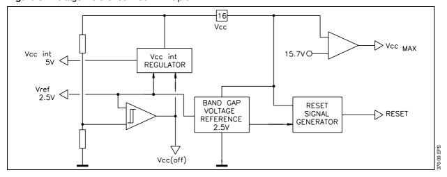
Figure 10: Operating Principle
