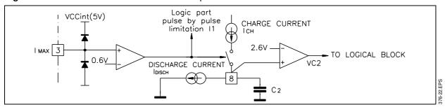
Two actions are carried out when the first threshold is reached
