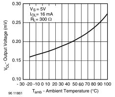
Figure 7. Output Voltage vs. Ambient Temperature
