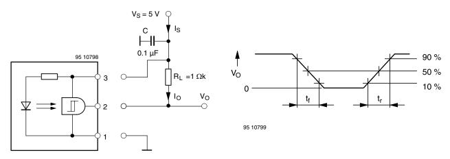
Figure 1. Test circuit and pin connection
