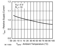
Figure 5. Rel. Supply Current vs. Ambient Temperature
