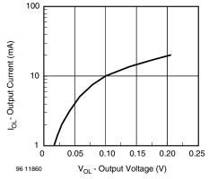
Figure 6. Output Current vs. Output Voltage
