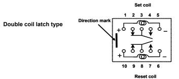
Double coil latch type (Reset position)
