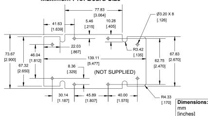
Enclosures can be Factory Modified (Milling, Drilling, Printing etc.) Contact Factory mjm@hammondmfg.com for quotes Solid models of this enclosure available in STEP or IGES. (Part number and text placement/orientation on our products are subject to change,
