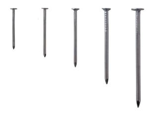
**Technical data:** 275 steel nails • Material: steel, material no. 1.0035 (Q195) • yield strength max. 195 MPa • tensile strength max. 430 N/qmm.
