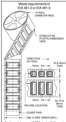
Each reel has a 15.750 inch (390 mm) minimum leader and a 6.30 inch (160 mm) minimum trailer.
