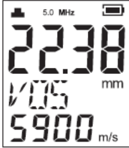
Well coupled, and in process of thickness measuring.
