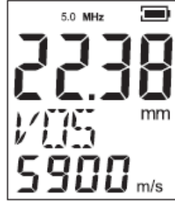
Thickness measuring completes, remove the sensor away.
