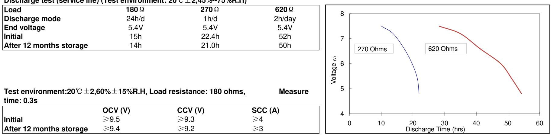
Remark: OCV: Open Circuit Voltage; CCV: Close Circuit Voltage; SCC: Short Circuit Current
