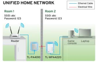
${}^{*}\mathsf{The}$  Powerline Adapters need to be connected in the same electrical circuit.
