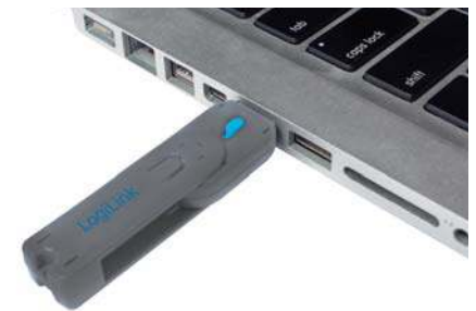
Insert the Key with blocker to an USB port
