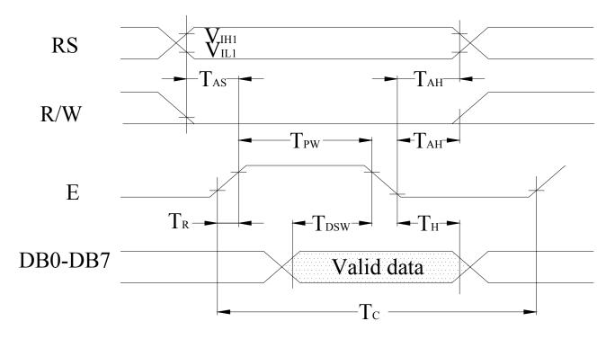
•Reading data from ST7920 to MPU
