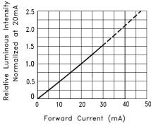
Fig.4 Relative Luminous Intensity vs. Forward Current
