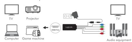
Ideal converter for YPbPr and Audio signals into HDMI signals
