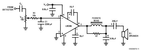
$\textbf{Note 4:} \ \, \textbf{Twist Supply lead and supply ground very tightly}.$
