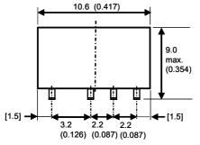
Tolerance of lead pitch is  $\pm 0.15 \text{mm}$  (0.006inch) Other tolerances  $\pm 0.3 \text{mm}$  (0.012inch)
