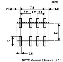
Tolerance of lead pitch is  $\pm 0.15$ mm (0.006inch) Other tolerances  $\pm 0.3$ mm (0.012inch) Lead size  $0.4x0.2 \pm 0.1$
