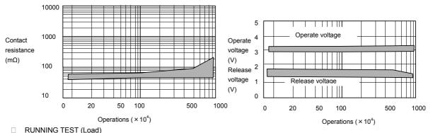
(Load: 50VDC 0.1A resistive, Drive:5V.DC, 5Hz, 50% duty, Ambient temperature:85°C, Sample:UA2-5NU, 10pieces)
