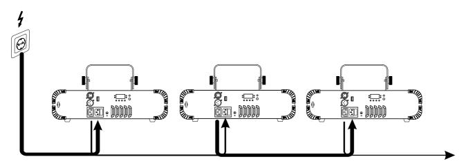
The device uses an auto-range power supply that accepts input voltages between 100 und 240 volts.
