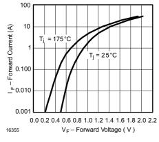
Figure 2. Forward Current vs. Forward Voltage
