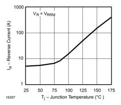
Figure 4. Reverse Current vs. Junction Temperature
