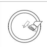
1. Power off, tap the central area of the diffusion plate with a pointed tool, and take out the cracked diffusion plate
