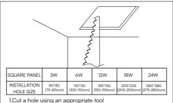
1.Cut a hole using an appropriate tool according to the cut-out size.
