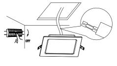
2.Switch OFF the power & Connect AC: 220-240V voltage with terminals.
