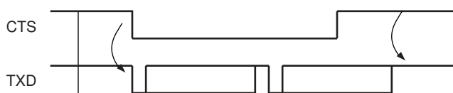
Figure 36-28. Transmitter Behavior when Operating with Hardware Handshaking
