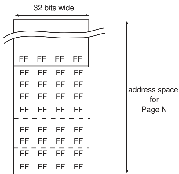
Step 1: Flash array after page erase
