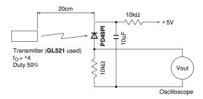
In the above figure, the transmitter should be set so that the output  $V_{out}$  can be  $40 \text{mV}_{P-P}$ .
