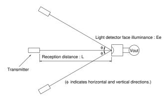
Fig. 2 Standard optical system
