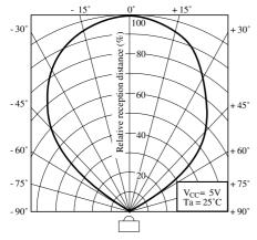
Fig. 2 Sensitivity Angle (Horizontal Direction)
